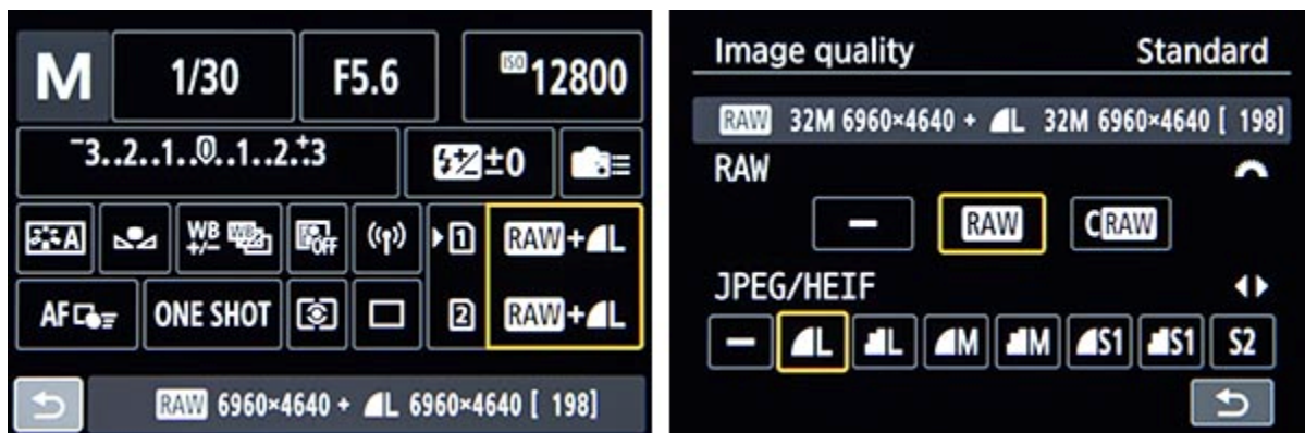
Figure 6.10 - Image Quality - Use the shooting settings Quick Control Screen (left) to access the Image Quality setting options (right). The Image Quality setting is used for selecting the RAW and the JPEG / HEIF file format, and the desired quality to save your image files. Turn the top Main Dial to select the RAW option, and use the left and right Cross Keys to select the JPEG / HEIF option, as indicated by the icons on the right side of the screen.
