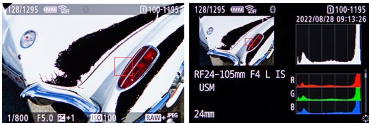
Figure 6.7 - Left: Large areas of white on the car have been overexposed (due to the use of exposure compensation here), and thus the blinking Highlight Alert shows them mid-blink, in black. Right: The overexposed areas are also represented by the spike along the right side of the Brightness Histogram graph.
