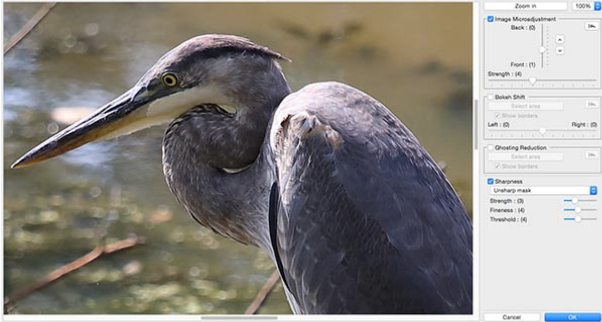
Figure 3.8 - The Dual Pixel RAW Optimizer window of Canon's Digital Photo Professional (DPP) software, showing the available adjustments at right.
