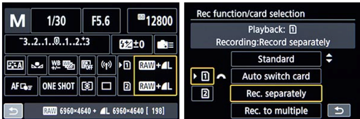
Figure 3.5 - You can also use the shooting settings Quick Control Screen to change the Image Quality Settings (left), as well as the related Record Function / Card Selection setting (right).
