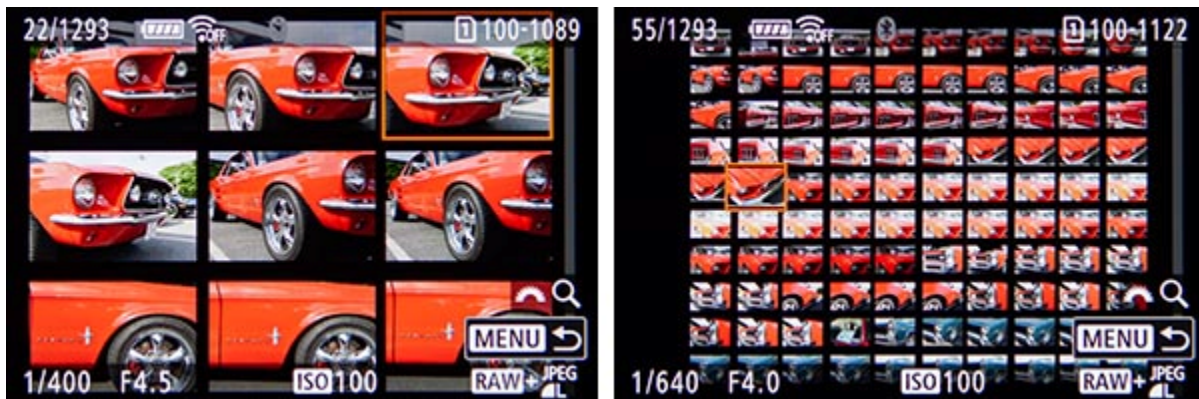
Figure 6.2 - Image Playback - Left: Zoom-out during image playback to view an index screen with multiple images. Right: Continue to zoom-out to view up to 100 thumbnails.
