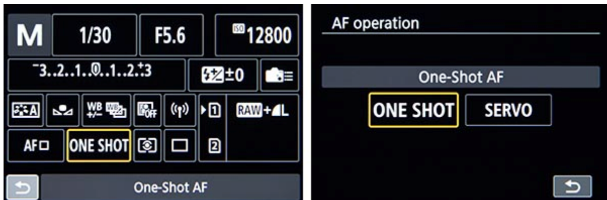
Figure 7.4 - Left: The Quick Control Screen with the AF Operation icon highlighted. The AF Area icon is just to the left of the AF Operation icon. Change the setting directly on the screen by turning a dial, or press the Q / SET Button and make your selection (right).
