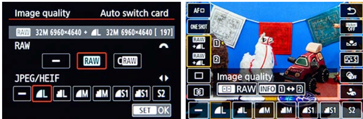
Figure 3.4 - Image Quality Settings - Left: Select the desired RAW format and/ or the highest quality JPEG format. Right: Accessing the Image Quality settings on the Live View Quick Control Screen. On the Live View screen, press the AF Point Selection Button to choose the RAW Image Quality.
