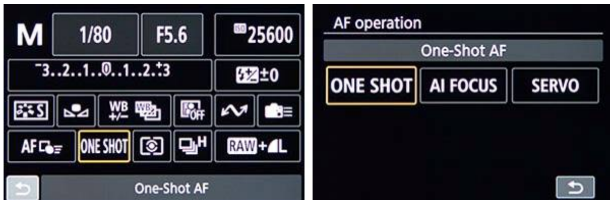
Figure 7.4 - Left: The Quick Control Screen with the AF Operation icon highlighted. The AF Area icon is just to the left of the AF Operation icon. Change the setting directly on the screen by turning a dial, or press the SET Button and make your selection (right).
