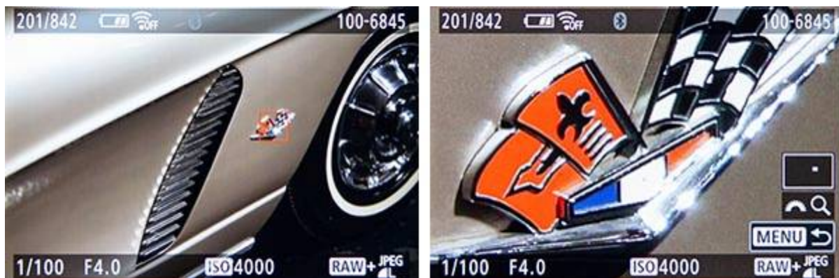
Figure 6.1 - Image Playback - Left: Press the Playback Button to view the captured images. Right: Press the Magnify Button and turn the top Main Dial to zoom-in and inspect the details and the focus of an image.
