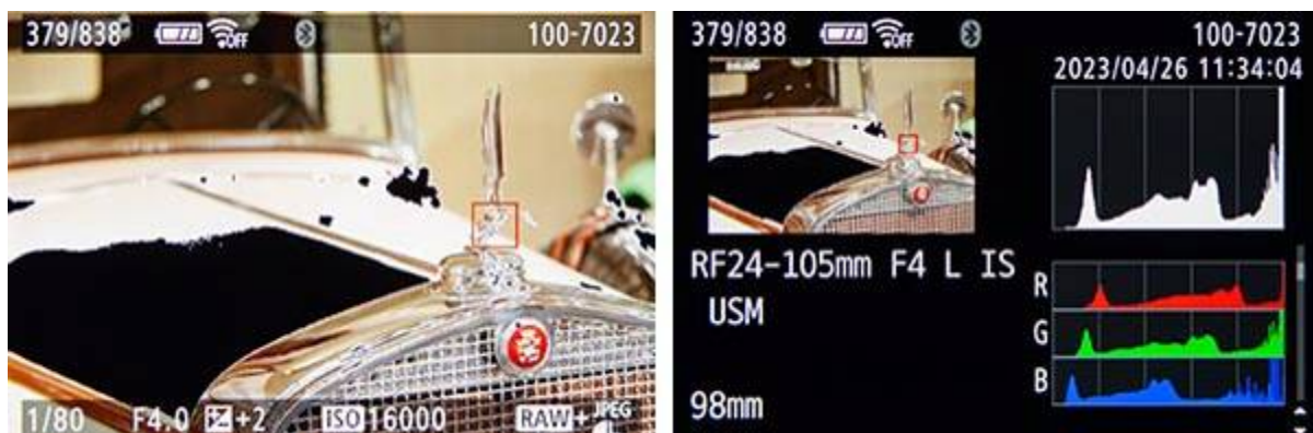
Figure 6.7 - Left: Large areas of the white car have been overexposed (due to the use of exposure compensation here), and thus the blinking Highlight Alert shows them mid-blink, in black. Right: The overexposed areas are also represented by the spike along the right side of the Brightness Histogram graph.
