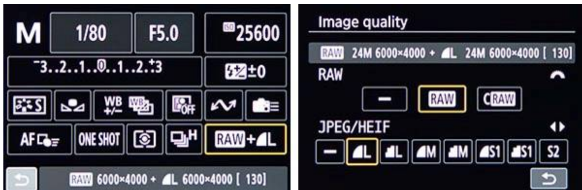
Figure 6.10 - Image Quality - Use the shooting settings Quick Control Screen (left) to access the Image Quality setting options (right). The Image Quality setting is used for selecting the RAW and the JPEG / HEIF file format, and the desired quality to save your image files. Turn the top Main Dial to select the RAW option, and use the left and right Cross Keys (or the top-rear Quick Control Dial) to select the JPEG / HEIF option, as indicated by the icons on the right side of the screen.
