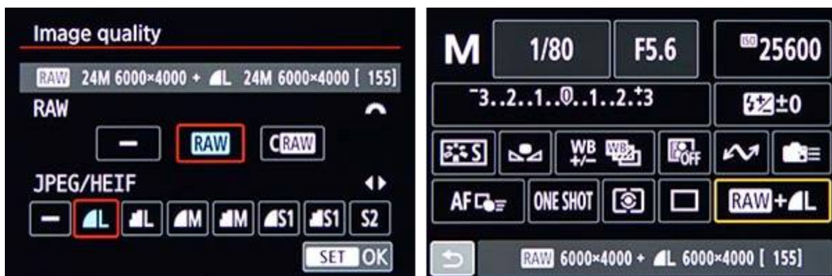
Figure 3.5 - Image Quality Settings - Left: Select the desired RAW format and/ or the highest quality JPEG format. Right: You can also use the shooting settings Quick Control Screen to change the Image Quality Settings.
