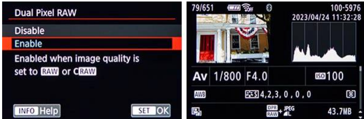
Figure 3.7 - Left: Enabling Dual Pixel RAW. Right: An image captured with Dual Pixel RAW, as shown on the Shooting Information Display during playback, as indicated by the "DPR" at the lower center of the screen.
