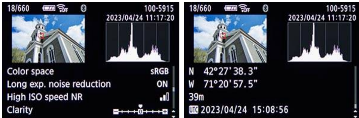
Figure 6.6 - Image Playback - Shooting Information Display, with additional camera settings (left), and with GPS information from a connected smartphone (right).
