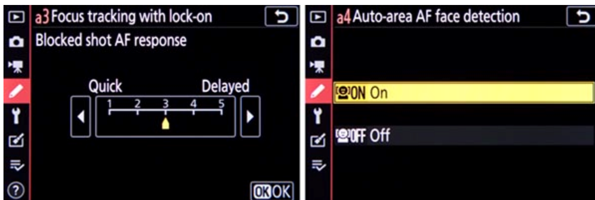
Figure 3.55 - Left: Focus Tracking With Lock-On settings - When working in AF-C Focus Mode and tracking a subject, this setting determines how long the camera waits before refocusing on a subject at a different distance. Right: Auto-Area AF Face-Detection item, to enable face-detection when using Auto-Area AF-Area Mode.
