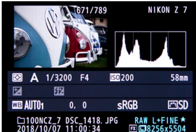
Figure 3.4 - The Overview information display screen during image playback, showing a thumbnail of the image, the combined RGB Histogram, and shooting and file information.
