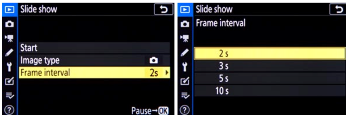
Figure 3.9 - Slide Show menu (left), used to select if stills and/or movies are shown, and how long each image is displayed (right).
