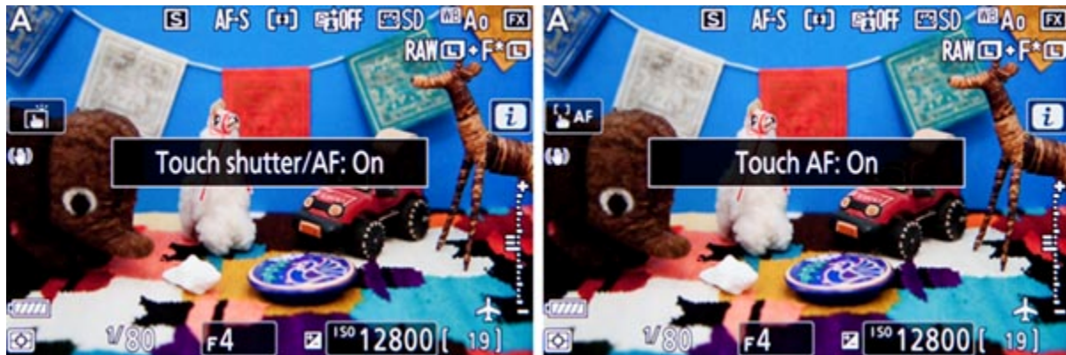
Figure 5.3 - Repeatedly tap the Touch Shutter icon (on the left side of the screen) to enable its different options. Left: Here it is being set for “Touch Shutter/AF: On”, which will enable you to tap the screen to focus and release the shutter. Right: The “Touch AF: On” setting will allow you to focus by tapping the screen, but the shutter will not be released.
