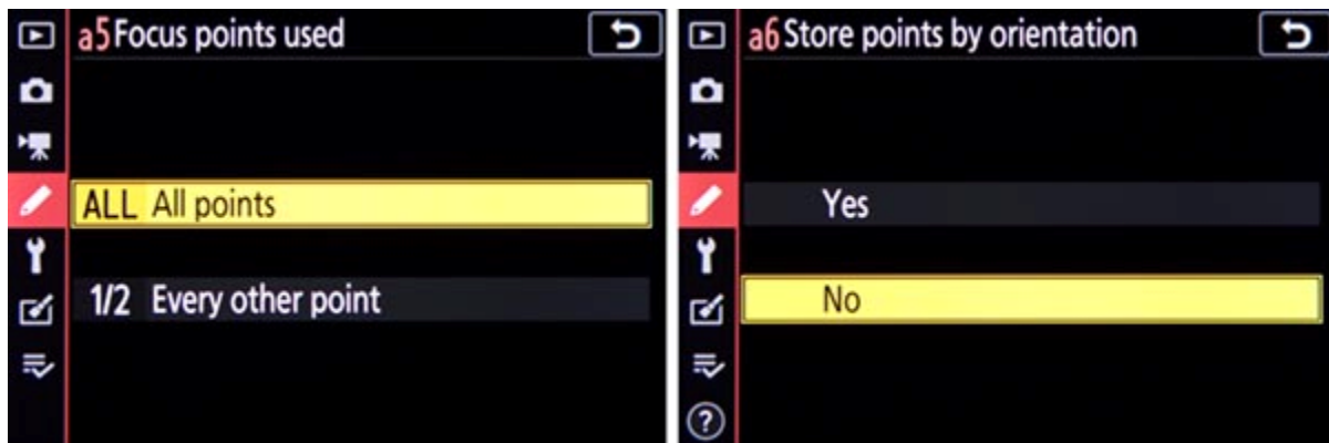
Figure 3.56 - Left: Number of focus points, to choose if All Points are selectable, or if Every Other Point is selectable. Right: Store Points By Orientation, to choose if the camera remembers the last focus point and/or AF-Area Mode used when the camera is held in a specific orientation.
