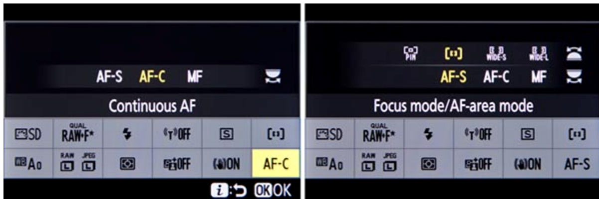
Figure 5.5 - Left: Or after highlighting the Focus Mode icon on the i Menu, turn the rear Main Command Dial to view and change the setting. Right: If you assign one of the Fn Buttons to the "Focus Mode/AF-Area Mode" option, you can press that button and turn the Command Dials to view and change those settings on the rear Monitor or in the
