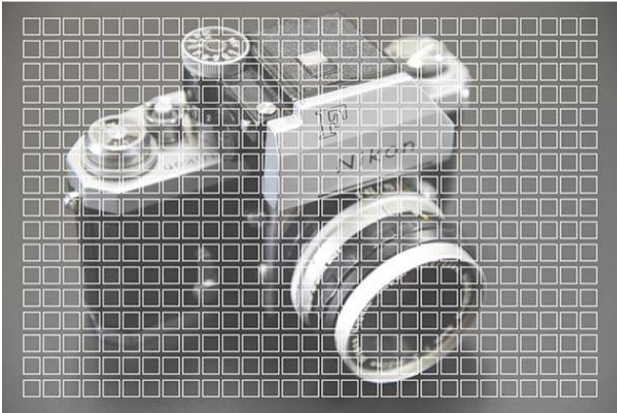
Figure 5.2 - Simulated view of the Nikon Z 8 Viewfinder, showing the location of all 493 AF Points. Note that you will not actually see all 493 AF Points in the Viewfinder or on the Monitor, only the active point or area.
