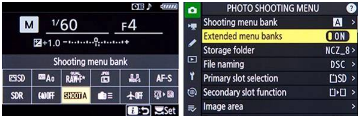
Figure 3.3 - Left: Shooting Menu Bank as seen on the Photo Shooting i Menu. Right: Enabling the Extended Photo Menu Banks, so that some additional shooting settings are also saved in the Banks.
