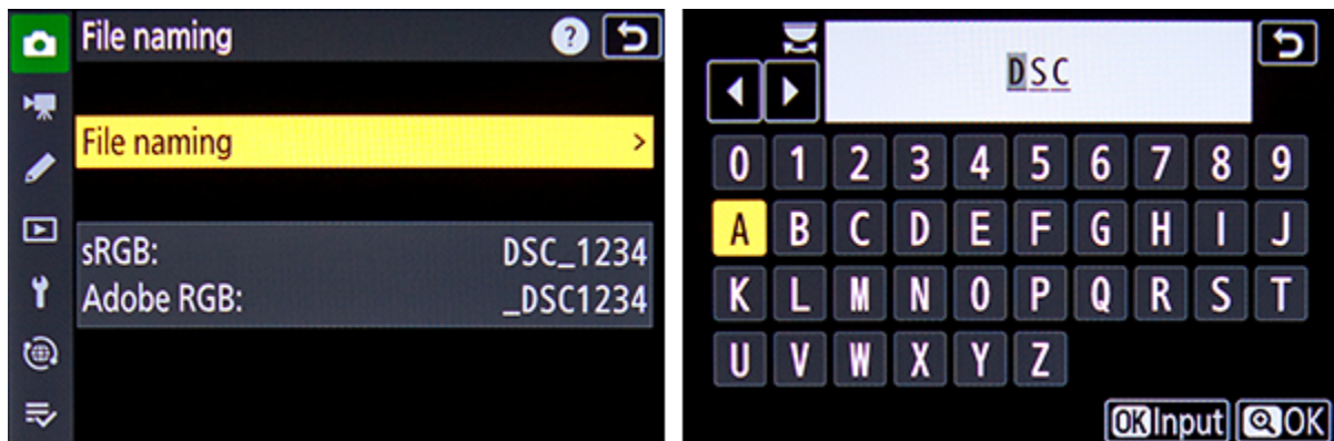
Figure 3.5 - File Naming menu (left), to change the “DSC” file name prefix if desired (right).
