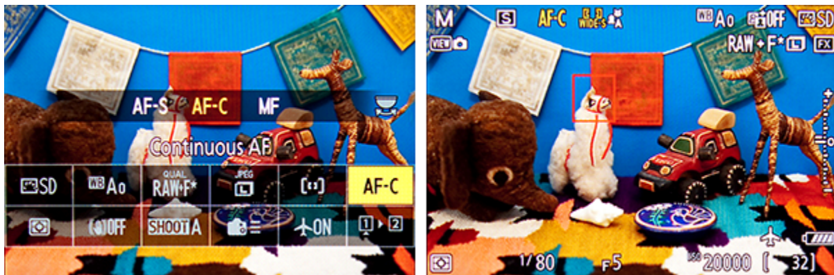
Figure 5.5 - Left: Or after highlighting the Focus Mode icon on the i Menu, turn the rear Main Command Dial to view and change the setting. Right: Or you can press the Focus-Mode Button on the front of the camera and turn the Command Dials to view and change those settings on the rear Monitor or in the Viewfinder. Use the rear Main Command Dial to change the Focus Mode and the front Sub-Command Dial to change the AF Area Mode. Here the Focus-Mode Button is being pressed and so the AF settings are seen in yellow at the top of the screen.
