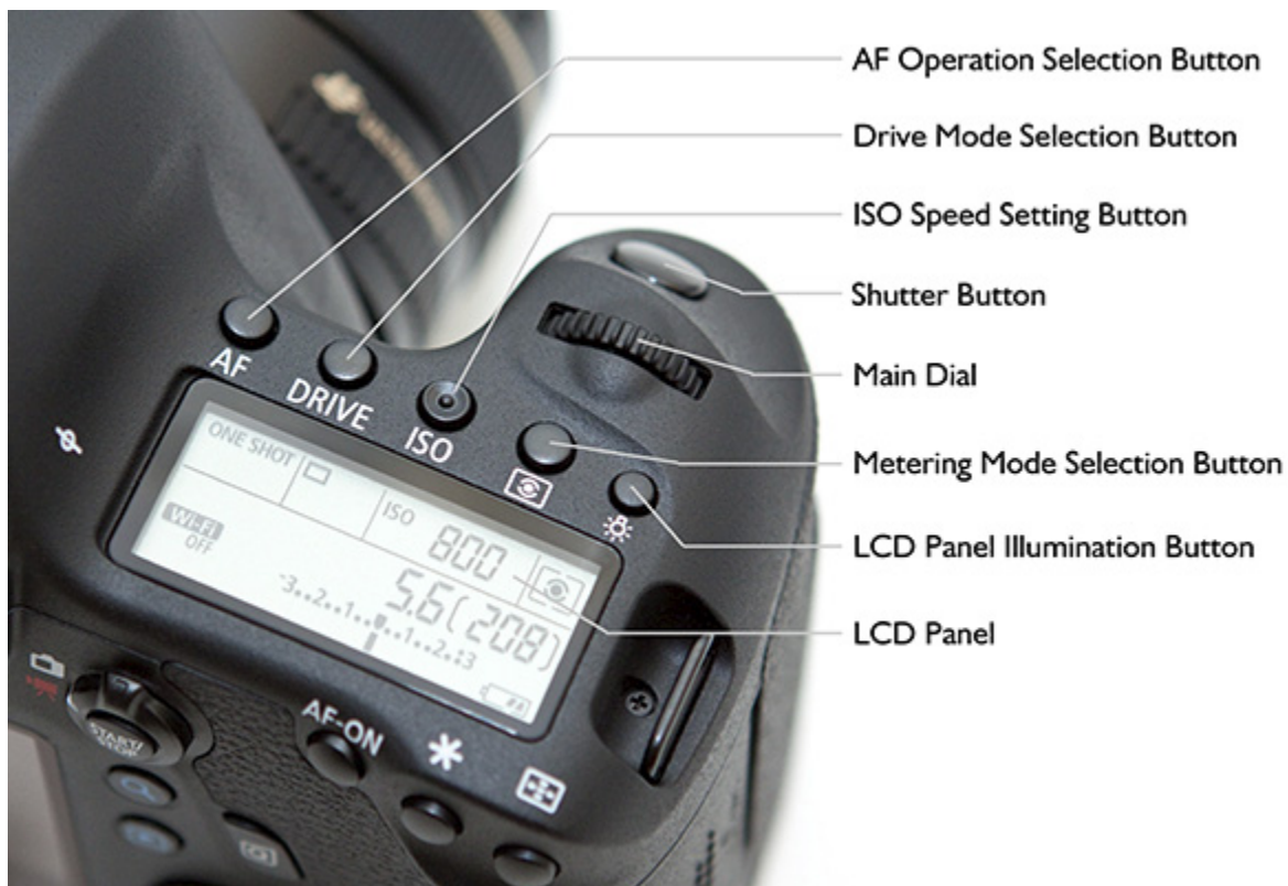
Figure 8 - Detail of the controls on the top of the Canon EOS 6D body.
