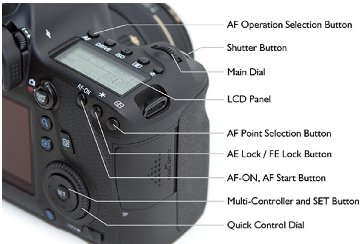
Figure 107 - Autofocus related controls of the Canon EOS 6D.
