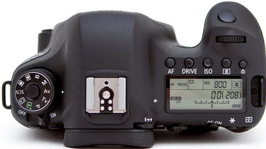
Figure 7 - View of the top controls of the Canon EOS 6D.
