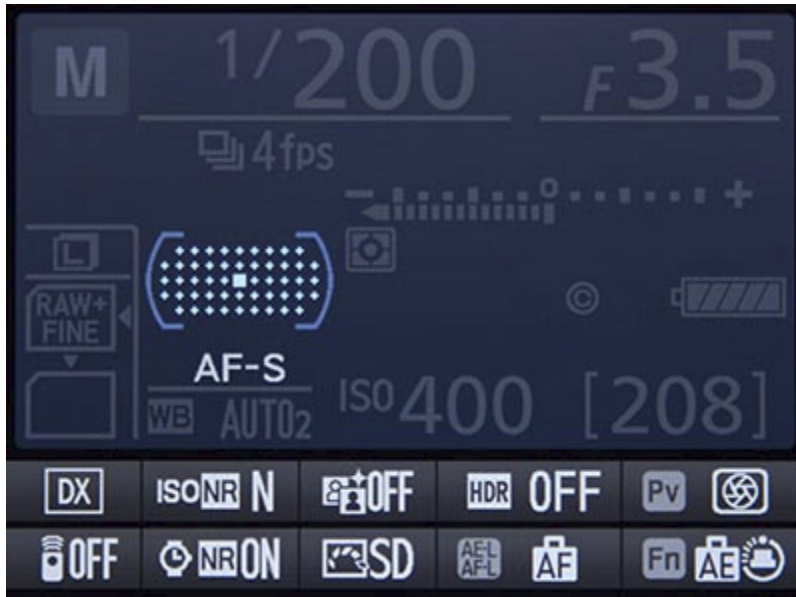
Figure 136 - Viewing and changing the Autofocus Mode and Autofocus AF-Area Mode on the rear Information Display, by pressing the AF-Mode Button and turning the Command Dials. AF-S and Single-Point AF shown here.
