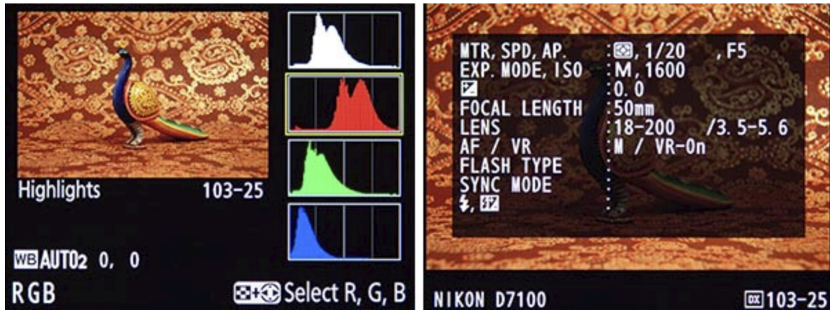
Figure 23 - RGB Histogram view during image playback (left). By pressing the Zoom-out Button and pressing right or left on the Multi Selector you can view the blinking highlights of the separate R, G, or B channels. The R-Red channel histogram is shown highlighted here. Right: Shooting Data view.
