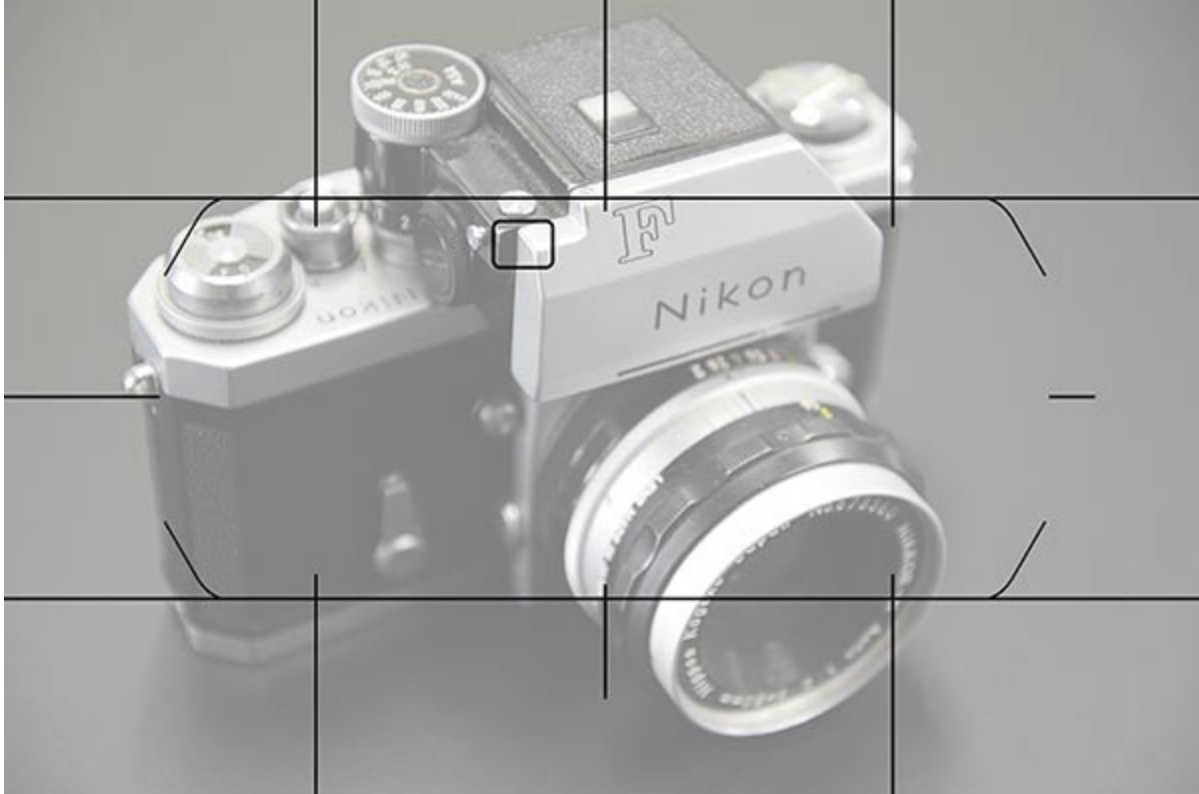
Figure 66 - Simulated view of Nikon D7100 Viewfinder, showing the optional Viewfinder Grid Display as well as a selected single Focus Point. Background image of Nikon F shown at 50% opacity to better see Viewfinder elements.
