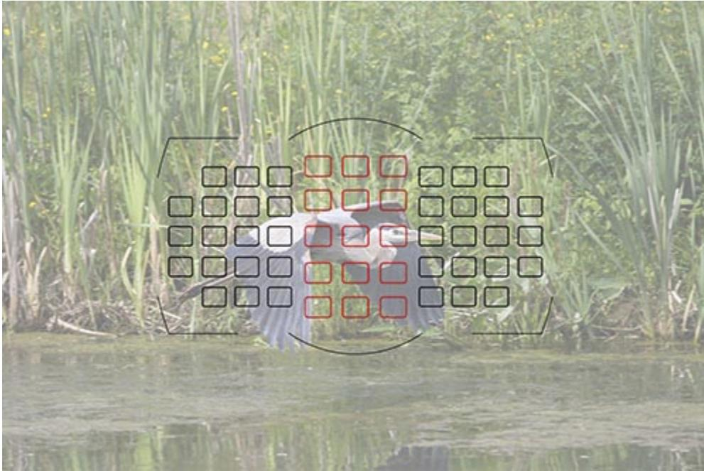
Figure 187 - Cross-Type Autofocus Points - The fifteen more sensitive cross-type AF points are shown here in red, located in the central area. (Simulated view of D810 Viewfinder, background image shown at 50% opacity. Note that all of the AF points will not actually be visible in the Viewfinder.)
