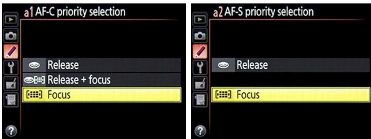
Figure 70 - Left: AF-C Priority Selection options, to determine if shutter release and maintaining the maximum continuous frame rate are the priorities, or if exact focus of each shot is the priority. Right: The similar AF-S Priority Selection options, for when working in AF-S Focus Mode.
