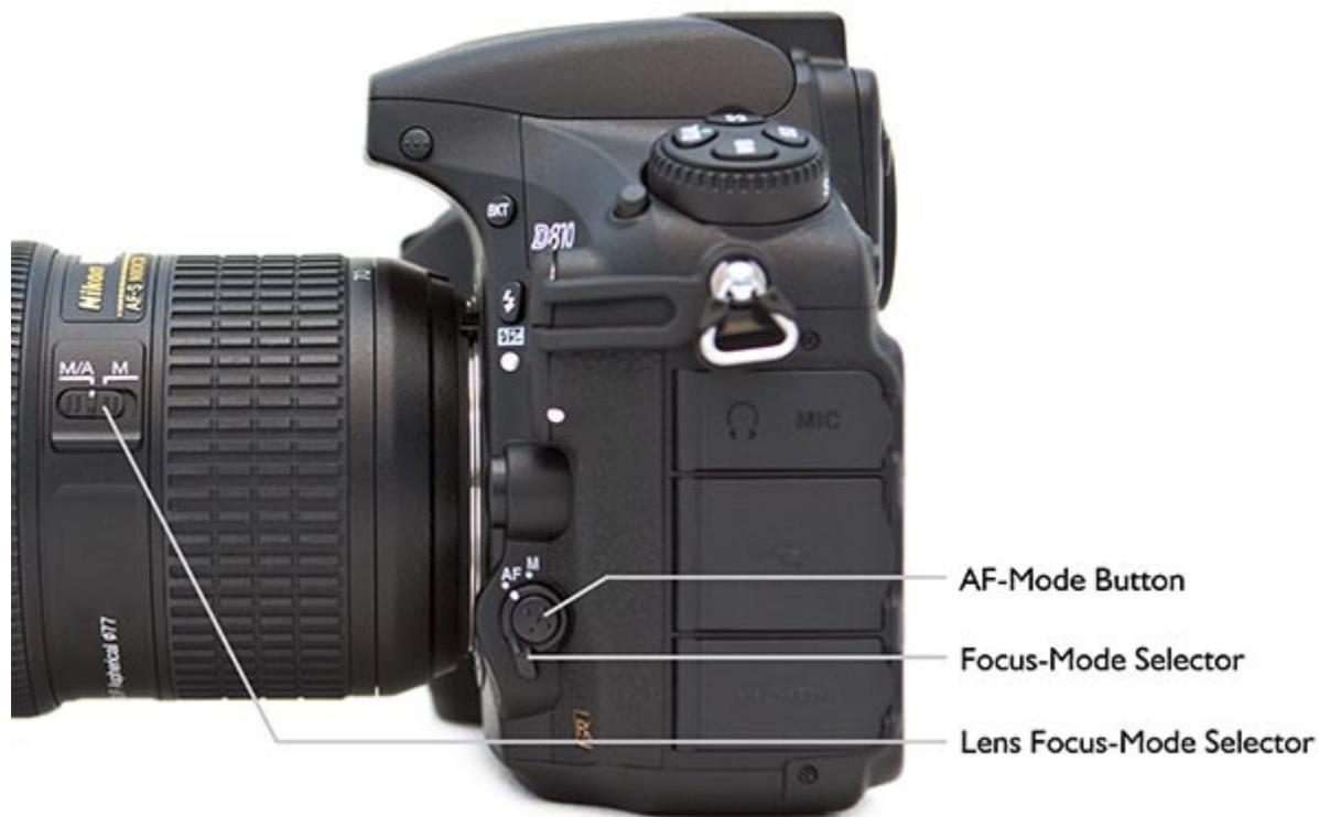
*Figure 189 - Additional autofocus controls of the D810.*
