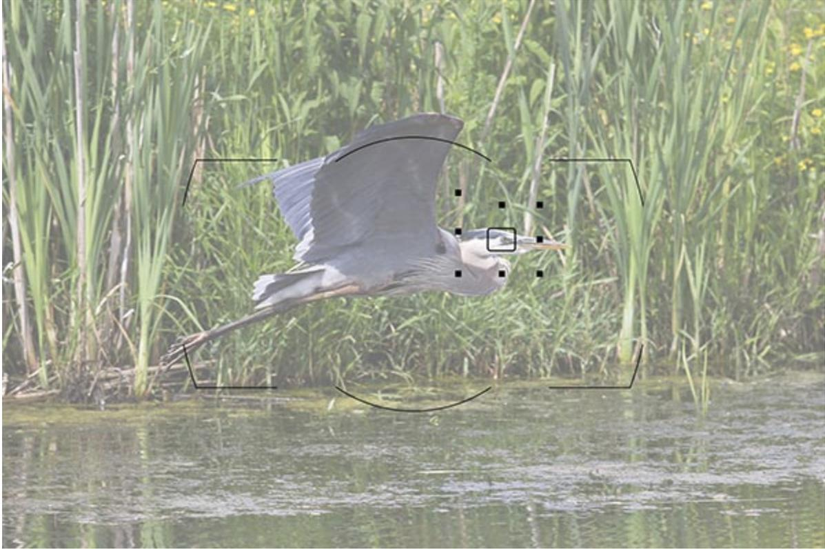
Figure 73 - Custom Setting a5: Focus Point Illumination - Simulated view of the D810 Viewfinder - Use the “Dynamic-Area AF Display” item of Custom Setting a5 to display just the single active AF point, or display all of the points of the Dynamic-Area, as shown here with 9-Point Dynamic Area. Background image shown at 55% opacity to better see Viewfinder elements. Shutter speed 1/1600, Aperture f/4.0, ISO 200.
