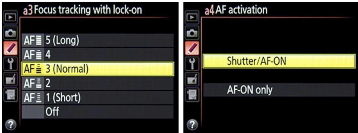
*Figure 71 - Left: Focus Tracking With Lock-On setting to determine how long the camera waits before refocusing on a subject at a different distance, when working in AF-C Autofocus Mode. Right: AF Activation options, to choose if the Shutter Button and/or the AF-ON Button initiates autofocus.*
