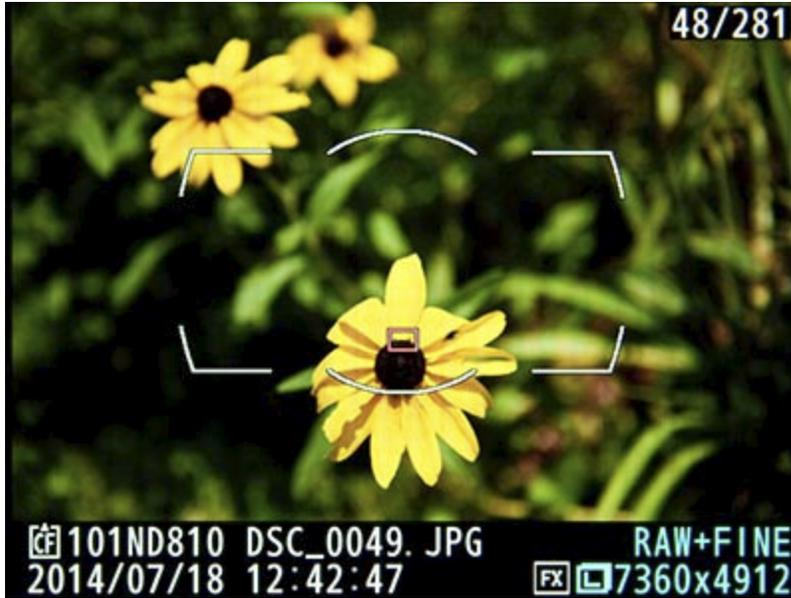
Figure 33 - File information view during image playback, with Focus point display enabled to show which Focus Point was used for autofocus with this shot, indicated by the tiny red square near the center of the flower.
