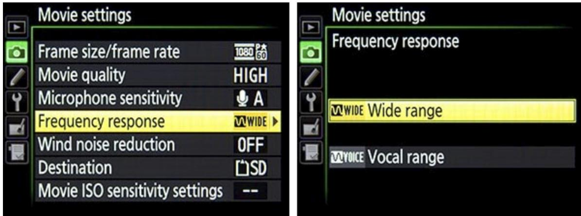
Figure 66 - Left: Movie Settings Menu used to choose movie options of frame size and rate, movie quality (maximum bit rate), audio settings, which memory card to use for saving movie files, and ISO settings. Right: The new Frequency Response option for the built-in or optional external mic.
