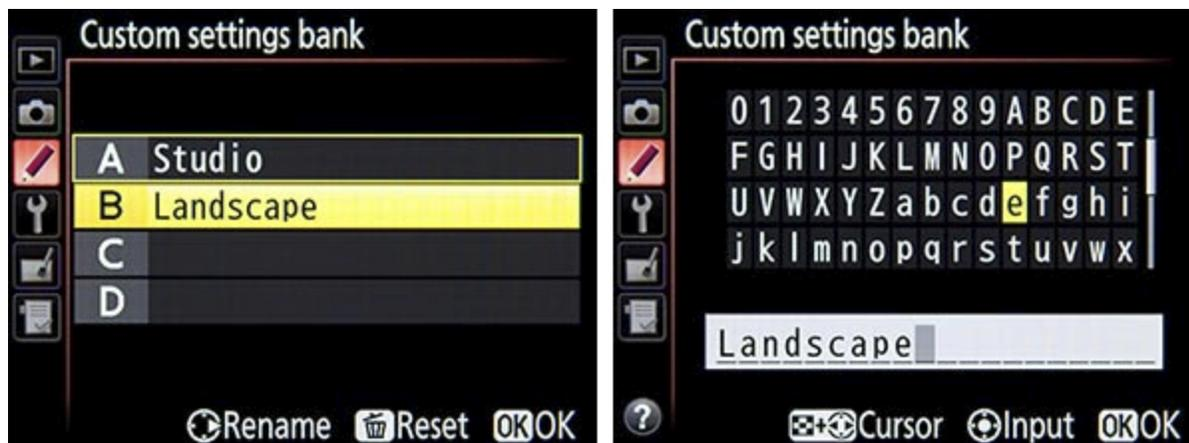
Figure 68 - Left: The Custom Settings Bank, allowing you to register and save a group of selected settings. Press right on the Multi Selector to name the Bank, as shown at right.
